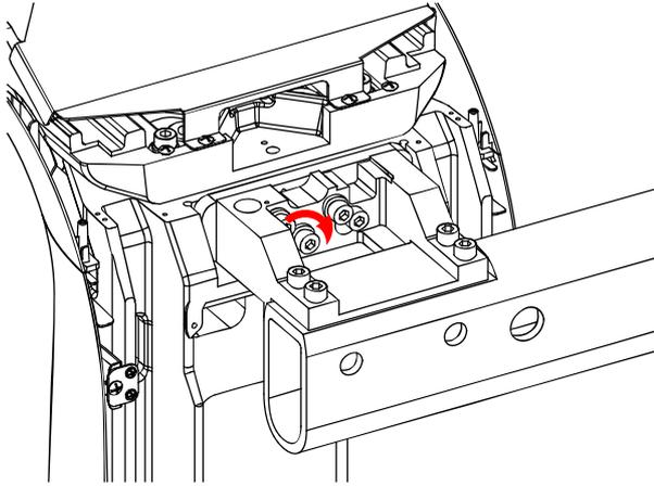
After the height adjustment of the One shot ceph (S) mechanism is complete, secure the M8x30 wrench bolt 4EA firmly.
