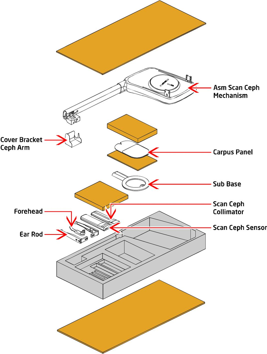
3.1.2 Scan Ceph Module Accessory
