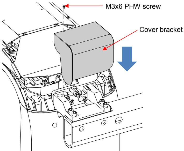
Insert the cover bracket into the connection between the Main body and one shot ceph(S) mechanism and assemble with M3x6 PHW screw 1EA.
