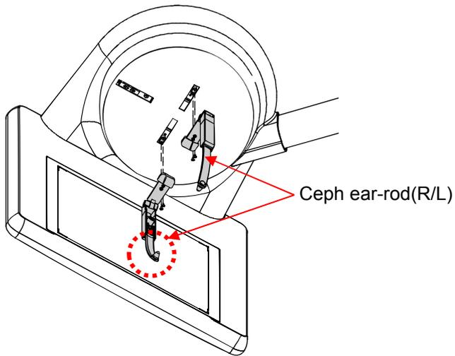
Assemble the ceph ear rod R/L with M4x12 wrench bolt(SEMS) 4EA.
