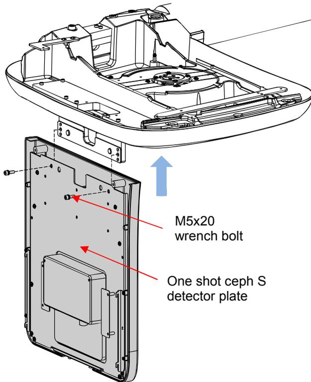
Assemble the one shot ceph(S) detector plate with the M5x20 wrench bolt 2ea.
