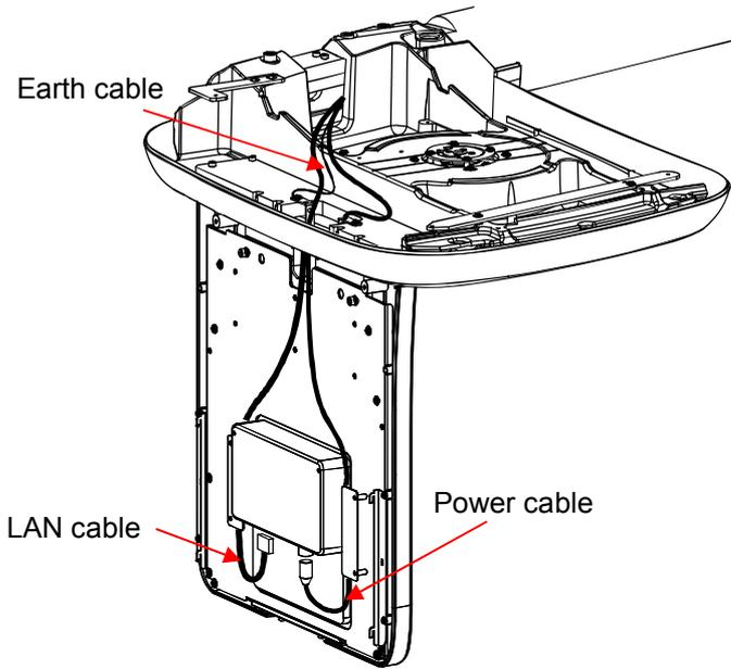
Connect cable of one shot ceph(S) detector as shown on the left.
