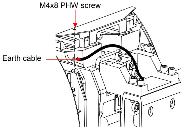
Secure Earth cable inserted into scan ceph mechanism onto the top of the Main body using M4x8 PHW screw.
