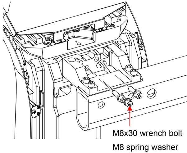
In order to fix the Scan Ceph mechanism attached to the body, be concluded loosen the M8 spring washer 3ea and M8x30 wrench bolt 3ea.
