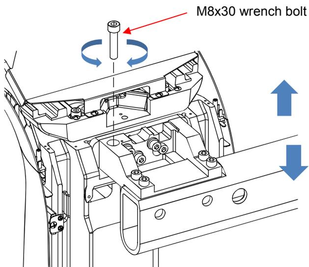
Assemble the M8x30 wrench bolt 1ea for level adjustment of the One shot ceph (S) mechanism.
