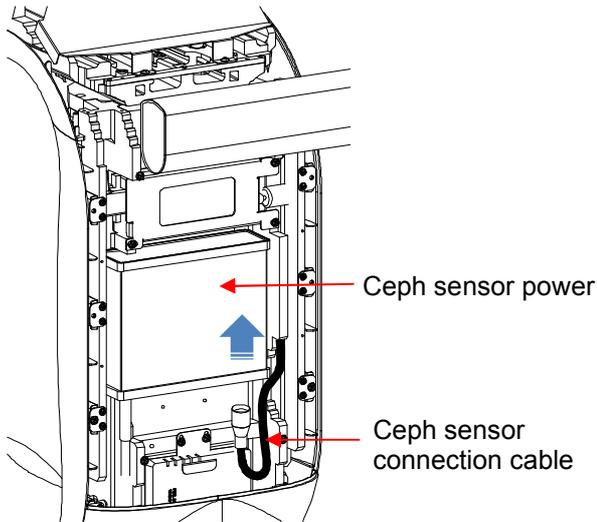
Insert the Ceph sensor connector cable inserted in the ceph mechanism into the ceph sensor power for connection. At this time, cable must pass through inside of the Power cover.
