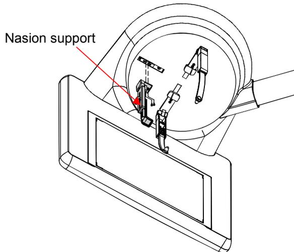
Assemble the nasion support with M4x12 wrench bolt(SEMS) 2EA.
