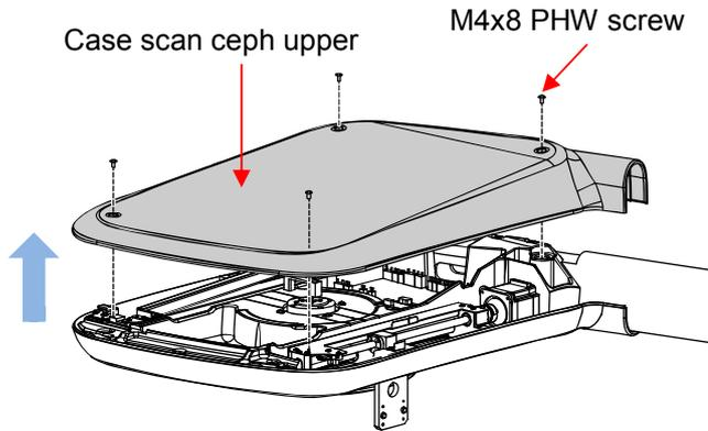
Unscrew M4x8 PHW screw 4ea and disassemble case scan ceph upper.
