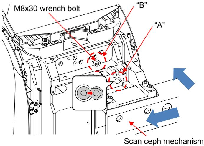
After you contact through the "B" portion of the M8x30 wrench bolt fixed to the arm fix sub plate part "A" hole of Scan Ceph mechanism, and install the scan ceph mechanism slide to the left.
