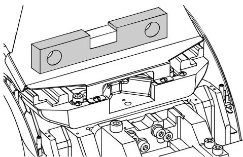
Use the level meter to check the level.
