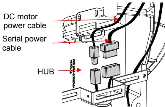
Connect serial power cable of scan ceph sub MCU board inserted in scan ceph mechanism and connector of scan ceph DC motor to connector of the body.
