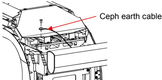
Use M4x8 PHW screw and M4 washer to fasten the ceph earth cable inserted in ceph mechanism to top of the main body.
