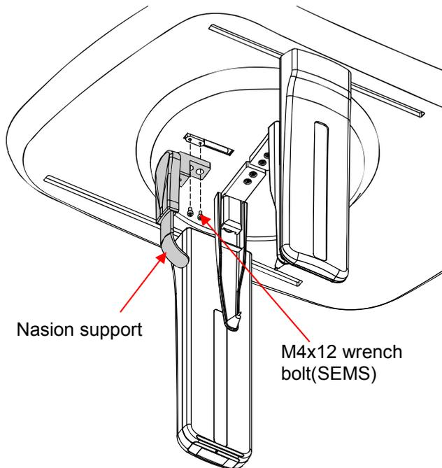
Assemble the Nasion Support with M4x12 Wrench Bolt(SEMS) 2EA.
