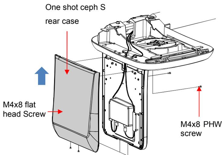
Assemble in M4x8 PHW screw 2ea and M4x8 flat head screw 2ea by assembling and slide hook so take upward from below one shot ceph(S) rear case.
