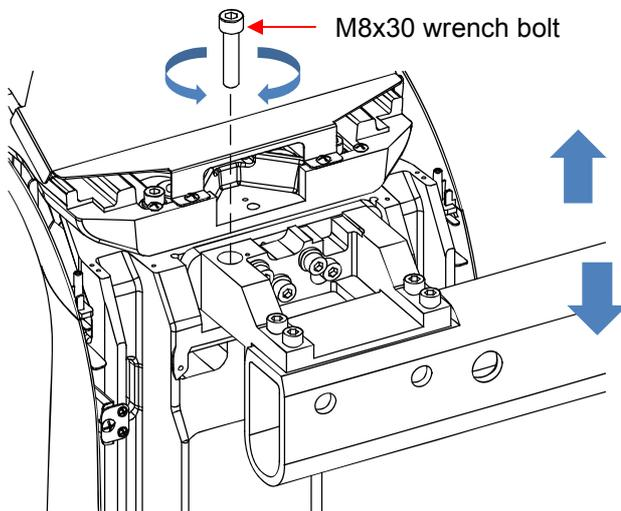
Assemble the M8x30 wrench bolt 1ea for level adjustment of the scan ceph mechanism.
