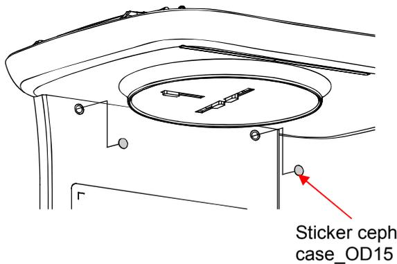
Attach the sticker ceph case\_OD15 2EA to the front case.
