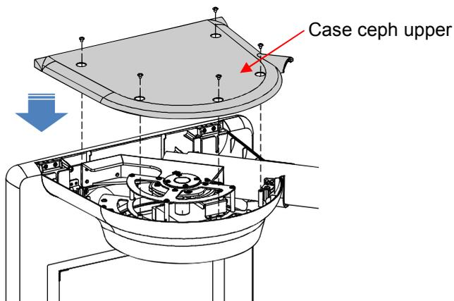
Assembly the case ceph upper with the M4x8 PHW screw 5EA.
