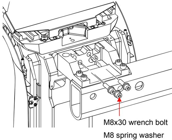
In order to fix the One shot ceph (S) mechanism attached to the body , be concluded loosen the M8 spring washer 3ea and M8x30 wrench bolt 3ea.
