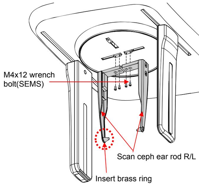
Assemble the Scan Ceph Ear Rod R/L with M4x12 Wrench Bolt(SEMS) 4EA.
