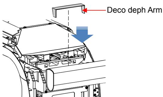
After Main body attachment of the Ceph Mechanism is completed, insert the Deco Ceph Arm.
