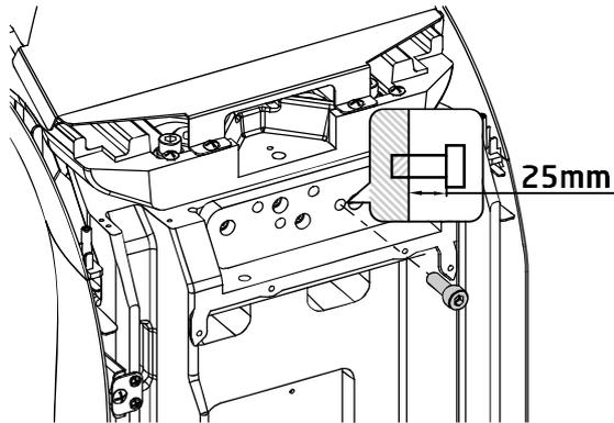
Assemble the M8x30 Wrench bolt to protrude about 25mm.
