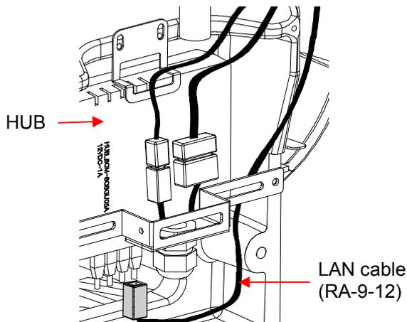
Connect LAN cable(RA-9-12) of sub MCU board inserted in scan ceph mechanism to HUB.
