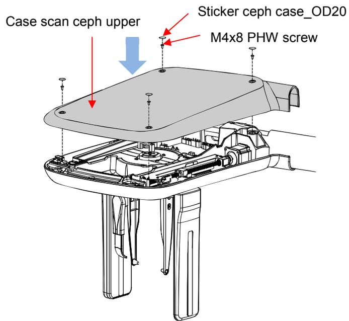
Assembly the Case Scan Ceph Upper with the M4x8 PHW screw 4ea and finish with Ceph Case\_OD20 sticker 4ea.
