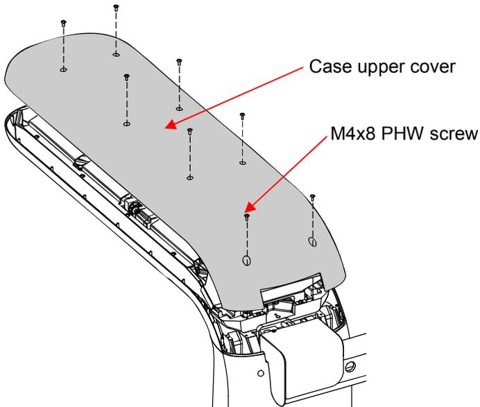
Assemble the Case Upper Cover with M4x8 PHW screw 8EA.
