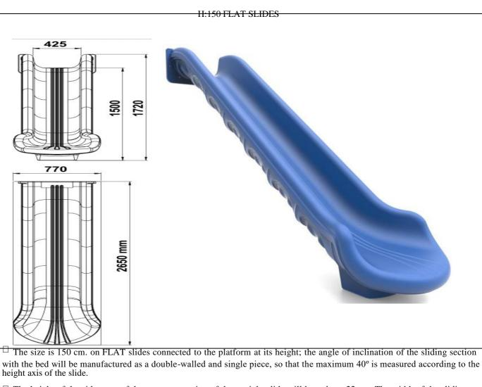
☐ The height of the side parts of the entrance section of the straight slide will be at least 22 cm. The width of the sliding
