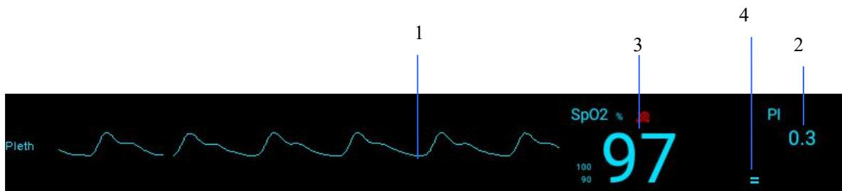
1. Pleth waveform (Pleth): visual indication of patient's pulse. The waveform is normalized.
