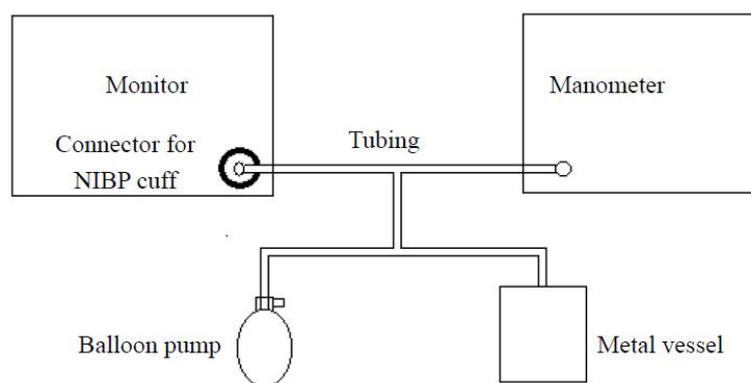
2. Before inflation, the reading of the manometer should be 0. If not, disconnect the airway and reconnect it until the readings is 0.
