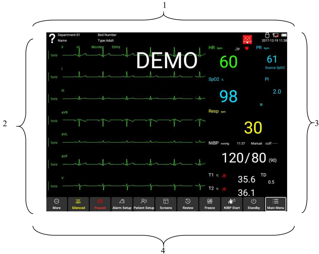
The monitor uses LED screen. It displays patient parameters, waveforms, alarm information, bed number, monitor state, date, time and some other information simultaneously.
