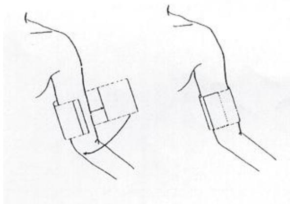
5. Connect the cuff to the air tubing and make sure that the bladder inside the cover is not folded and twisted.
