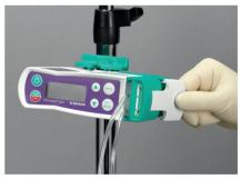
After loading the Enteroport<sup>®</sup> plus administration set and closing the pump door, the pump starts automatically activating all safety and control functions. This action is indicated on the display by the wheel sign rotating. After the process is completed, the pump can be started according to the (short) instructions for use.
