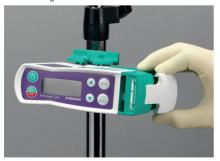
**3.** Slide the cassette of the administration set into the pump door track, check for correct fitting
