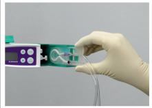
Close the door, close pump door mechanism
