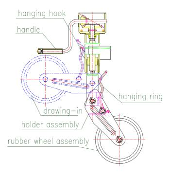
Fig.2-4 Schematic drawing of front guiding wheel structure
