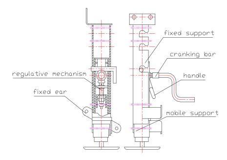
Fig. 2-5 Schematic drawing of supported leg structure
