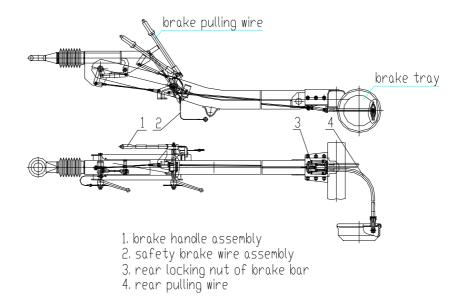
Fig. 2-3 Structure principle of the brake system
