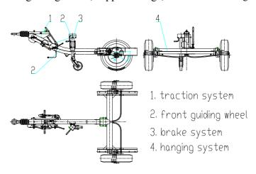
Fig.2-1 Chassis composition of the kitchen trailer
