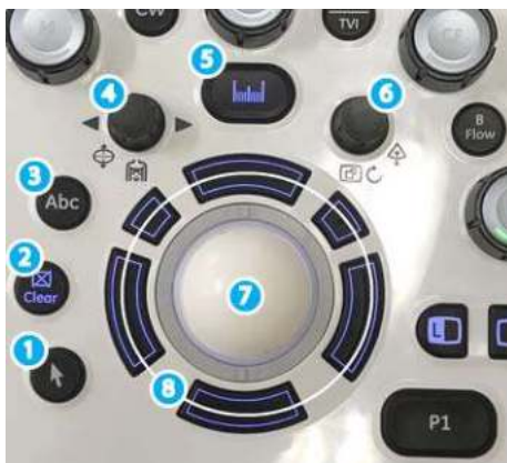
Figure 7-3. Measurement Controls on the Control panel
