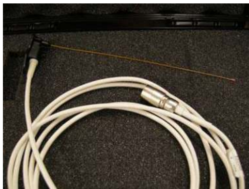
Figure 13-151. Needle Tip Sensor and Cable Close-up
