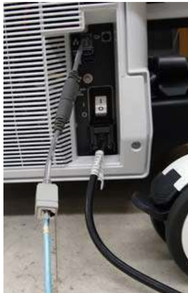
Figure 3-7. LAN cable with protection cable (example)
