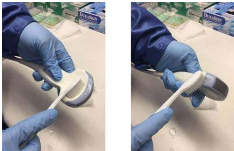
Figure 11-6. Cleaning the probe using a brush
