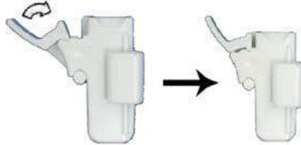
Figure 11-25. Locking the Needle Clip
