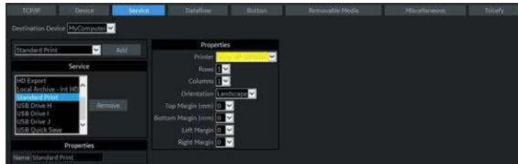
Figure 9-20. Connectivity -> Service Screen
