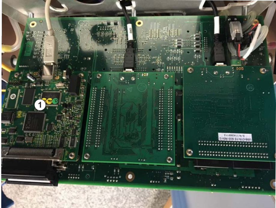
Fig. 5-105 Data acquisition board
