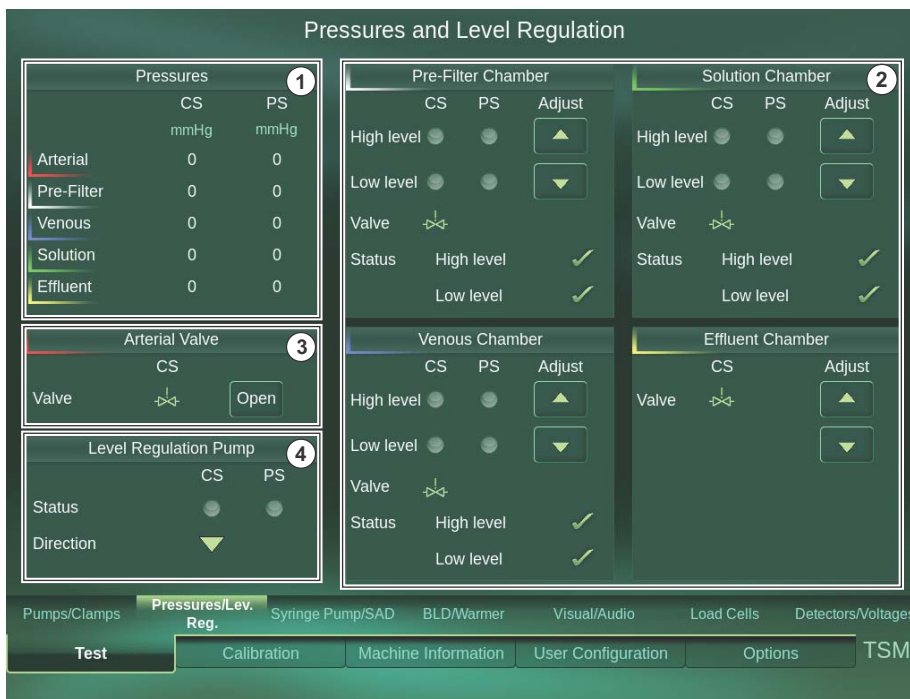
Fig. 6-18 TSM Test pressures and level regulation.
