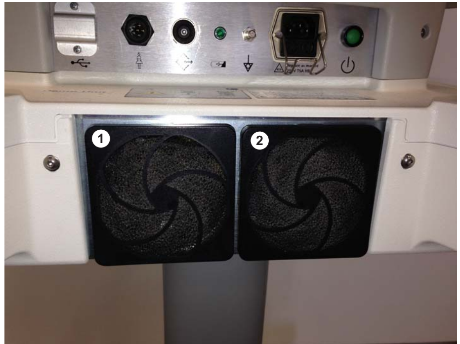
Fig. 5-128 Fan filter cover
