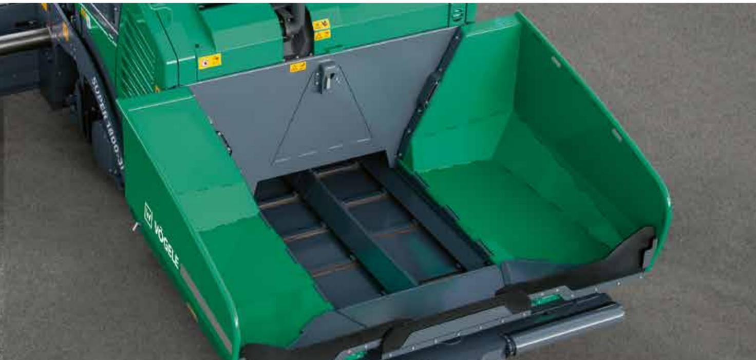
By spreading mix perfectly, the SUPER 1800-3(i) provides the ideal head of material in front of the screed in every paving situation.
