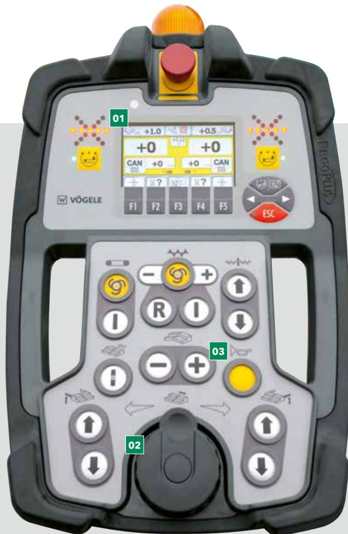
**01** The high-contrast colour display provides for brilliant readability even in poor lighting conditions. What's more, the downward-angled high-power LED lighting gives the operator a perfect view of all processes associated with the side plate, even in the dark.
