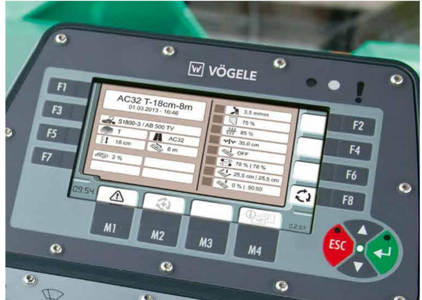
The Automatic function for paving programs allows an operator to create particular paving programmes. All the key parameters for paving a specific layer, e.g. a base course of asphaltic concrete 18 cm thick, can thus be stored.
