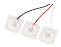
The prewired neonatal electrode are consist of a conductive adhesive hydro-gel, a Ag/ AgCl plated sensing element, a soft cloth or PE Foam substrate with the size of 22mm round and a 60 cm flexible tinned copper or carbon lead-wire terminating standard DIN connector.
