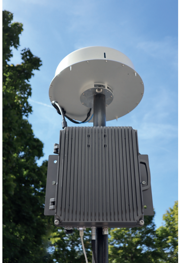
Fig. 1. The SignalShark Outdoor Unit and Automatic DF antenna for AoA and TDOA.
