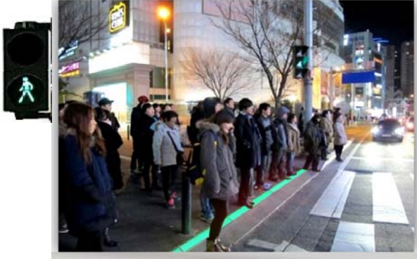
Corresponding with go signal of existing signal system, switching on the green light means enable to cross safety.
