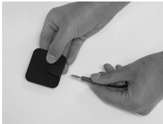
Figure 6.2. Connection of electrodes
