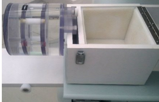
Figure 213. - Positioning the phantom
