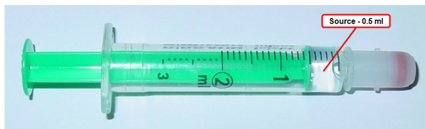
Figure 188. - Prepared syringe (closed with membrane adapter)
