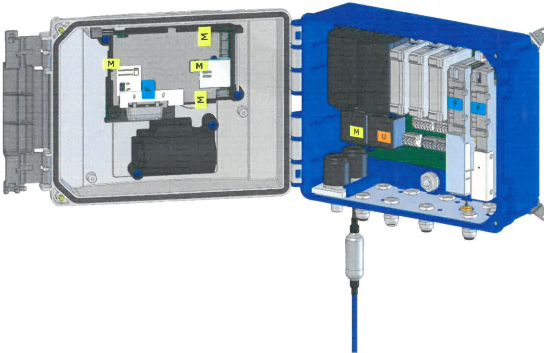
Figure no.6 Places of seals (stickers) on the conversion device of type ELCOR or ELCOR plus (version 1 - part 1)
