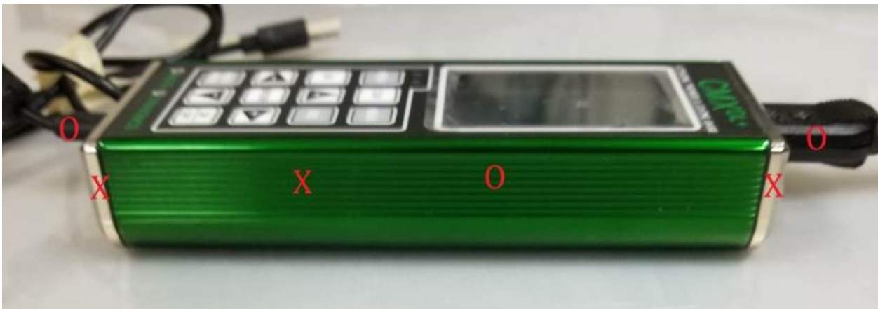
Photograph 5. ESD Test Points – Right of EUT
