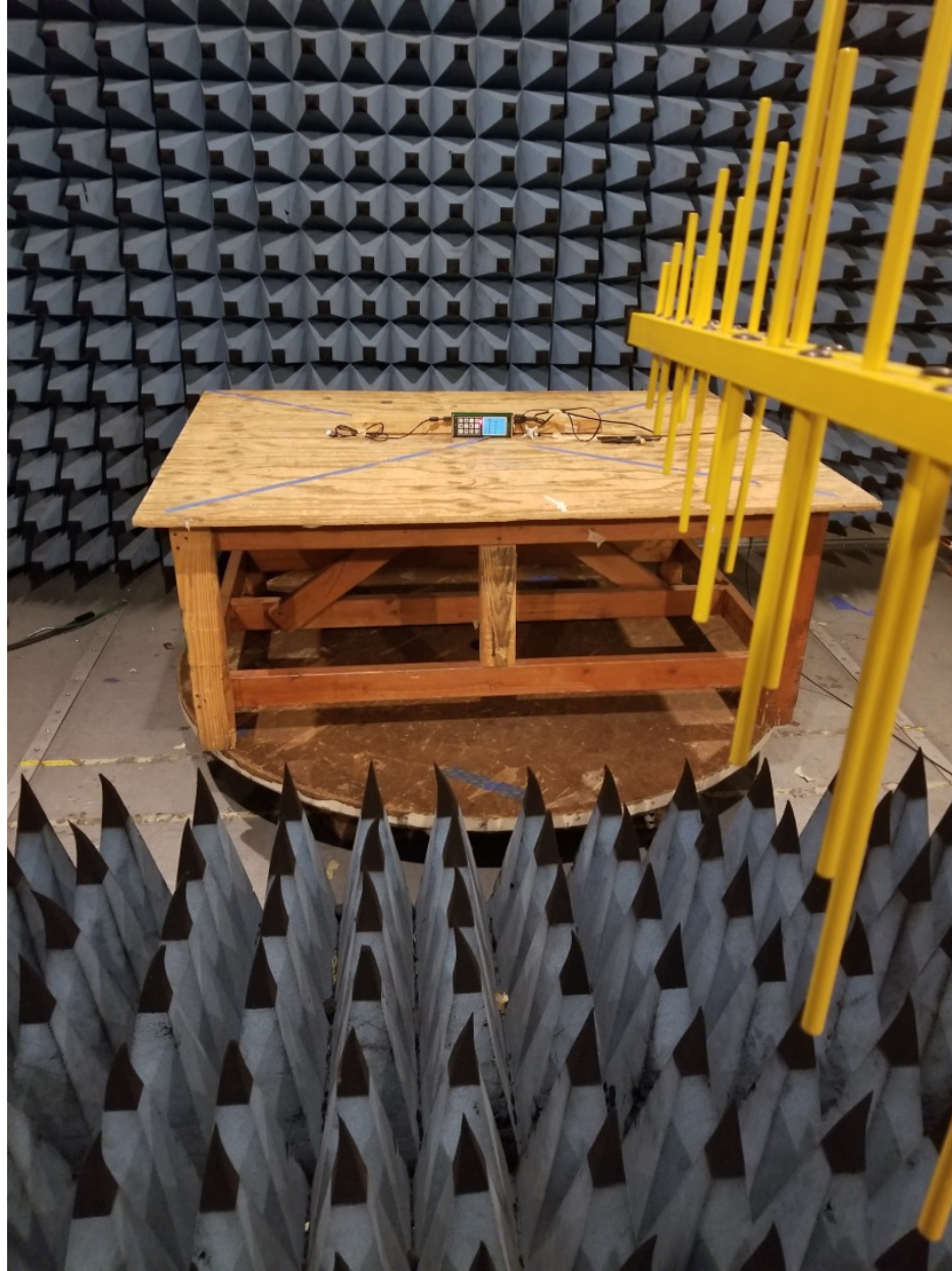
Photograph 10. RI (80 MHz – 1 GHz) Test Setup
