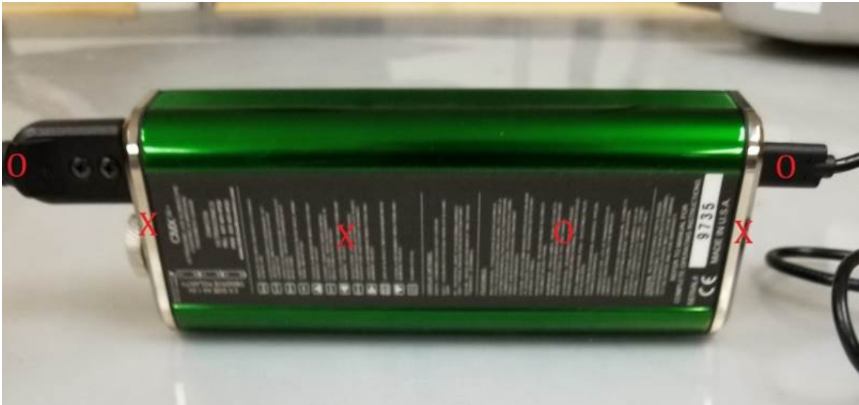
Photograph 4. ESD Test Points – Rear of EUT
