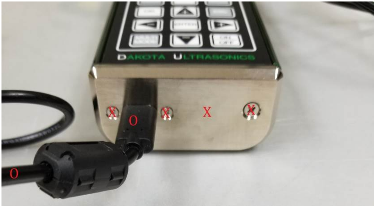
Photograph 8. ESD Test Points – Bottom of EUT
