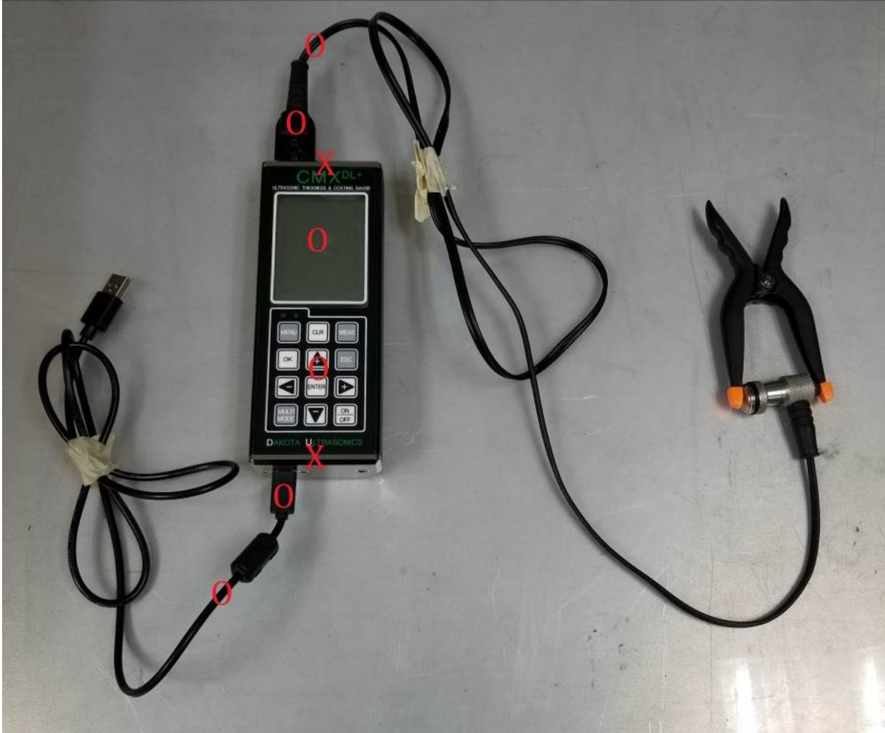
Photograph 3. ESD Test Points – Front of EUT
