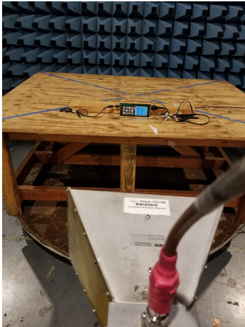
Photograph 11. RI (Above 1 GHz) Test Setup
