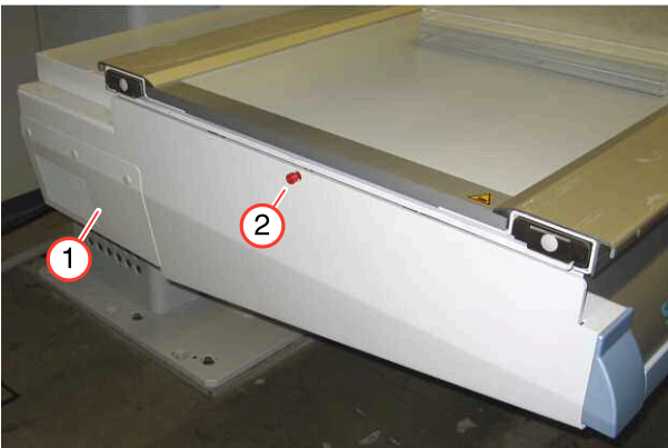
Fig. 26: Transport safety devices, left
