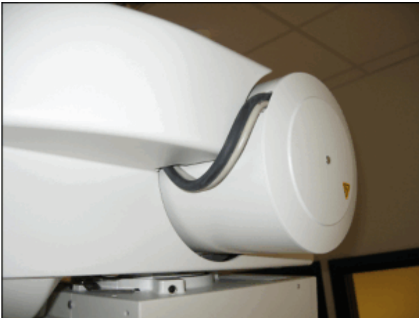
Fig. 108: Cable routing to the tube unit
