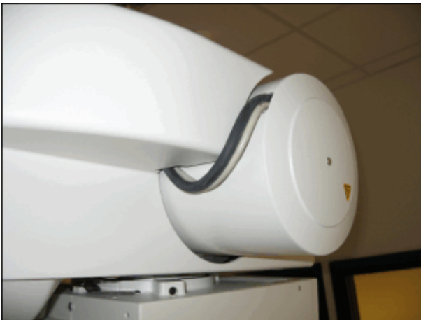
Fig. 49: Cable routing to the tube unit
