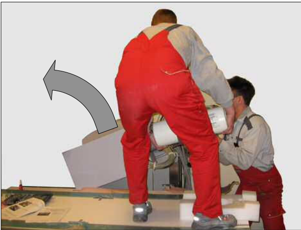
Fig. 30: Standing up the column
