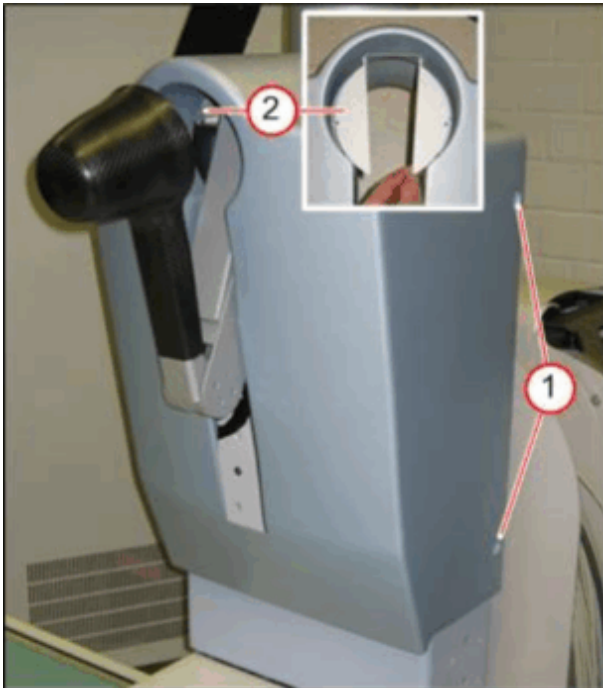
Fig. 128: Compression cover panel
