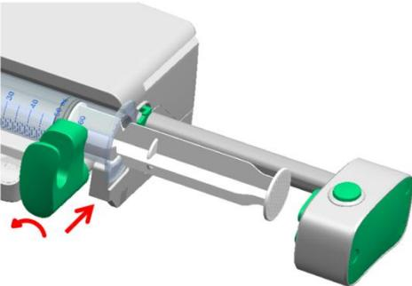
Step 5: Rotate the holder anticlockwise for 90° and release the holder.
