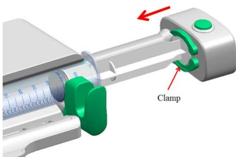
Step 6: The drive head automatically moves to the left until it withstands the syringe push-button, and the claw automatically clamps the syringe plunger.
