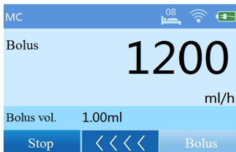
Manual bolus: During the infusion, tap and hold **Bolus** for 2s to start bolus. Keep on holding the button to continue bolus, and release the button to stop bolus. The pump automatically stops manual bolus when reaching the manual bolus limit even if the user keeps on holding the button.
