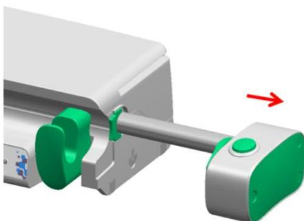
Step 1: Power on the syringe pump. The drive head automatically moves to the right.
