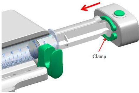
Step 6: Press and hold the clutch button, move the drive head to the left to withstand the syringe push-button, and release the clutch button.
