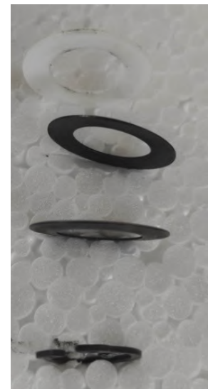
The 4 washers. From the top: Teflon washer, 2 conical washers, sieger ring
