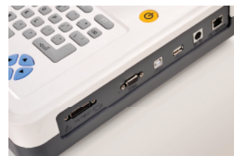
Memory of 300 patient records; USB memory storage; Network communication (RS232).
