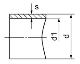
d = Tube outside diameter d1 = Tube inside diameter bar = Operation pressure at +23°C B.Radius = Min. bending radius
