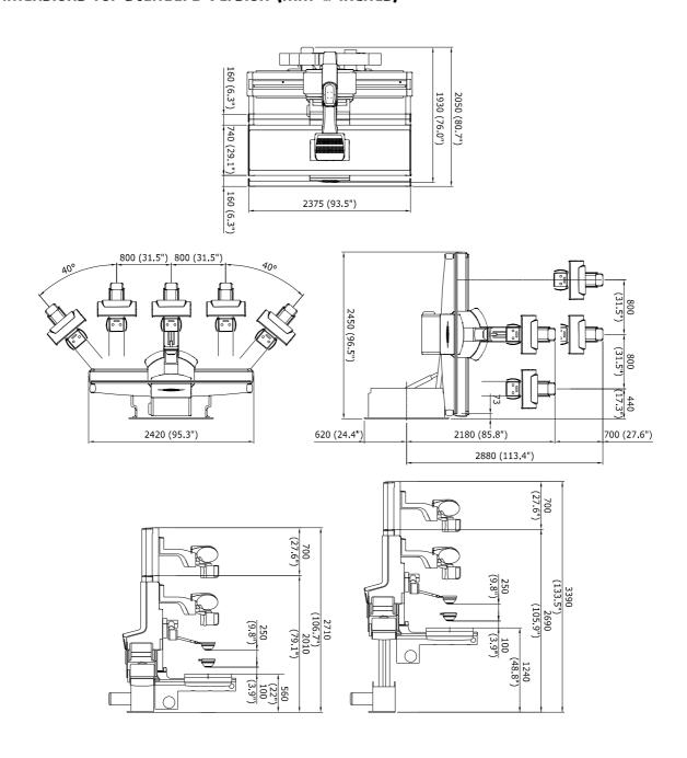
NOTE: Above measures are valid for installation with standard under-floor plate
