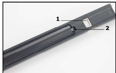
Figure 48: The test strip tray and its reference pad
