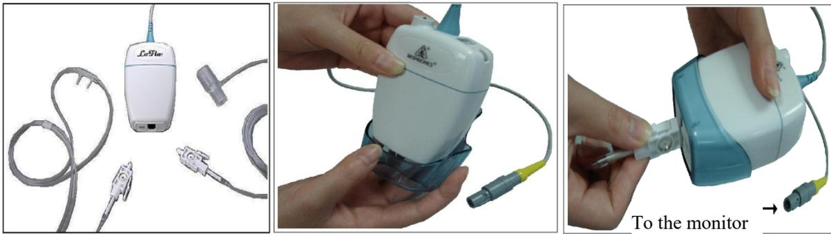
Fig 16-3 Respironics Sidestream CO<sub>2</sub> Connection Diagram
