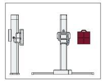
Floor-mounted solution with motorized Bucky wall stand equipped with Core XL for free exams
