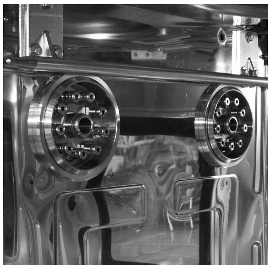
The channels connctons to the wash cart are inside the chamber on the left side (loading door)
