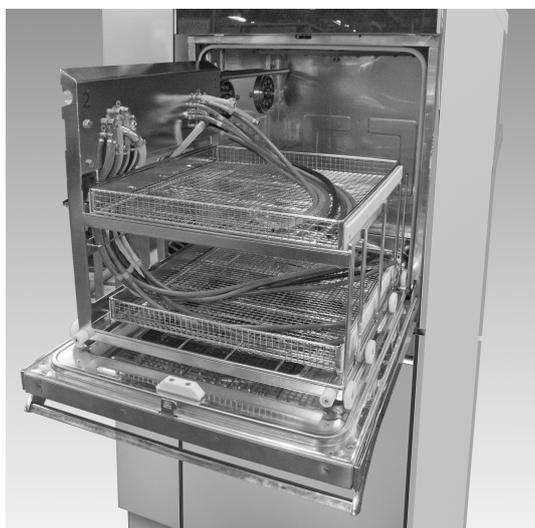
Open the device door. Pull out and remove the wash-cart
