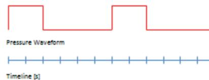
Breath number six and the following breaths are still pressure controlled breaths, and are regulated at the inspiratory pressure from the comparison of the set tidal volume versus the measured expiratory tidal volume.
