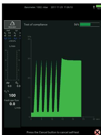
user is prompted to accept or reject. If the leakage is greater than 1000 mL/min the test will fail. Follow the instruction on the screen and repeat the test.
