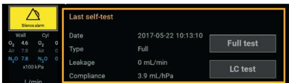
The values in this section are not editable but show details for the most recently performed self test of the machine. This information becomes part of the logged data for the patient case. For details about testing the machine as preparation for a procedure, see “Prepare the machine for use” on page 33.
