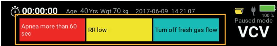
An alarm can be temporarily silenced by selecting *Silence Alarm* below the alarm area.
