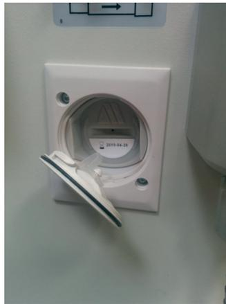
4. Insert the new O<sub>2</sub> fuel-cell sensor and close the interior lid.
