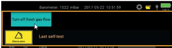
The top area of the screen can show patient alarms and technical alarms, for example, that the airway pressure is high. For details about changing default settings for alarms, see “Change default settings” on page 65.
