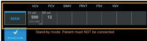
This section has a tab for each of the up to six automatic ventilation modes with the settings relevant for a mode displayed when the mode is selected. Use this section to prepare settings for a ventilation mode, or to start ventilation. For details about preparing a ventilation mode, see “Ventilation modes” on page 69. For details about settings during operation, see “Define ventilation settings” on page 44.
