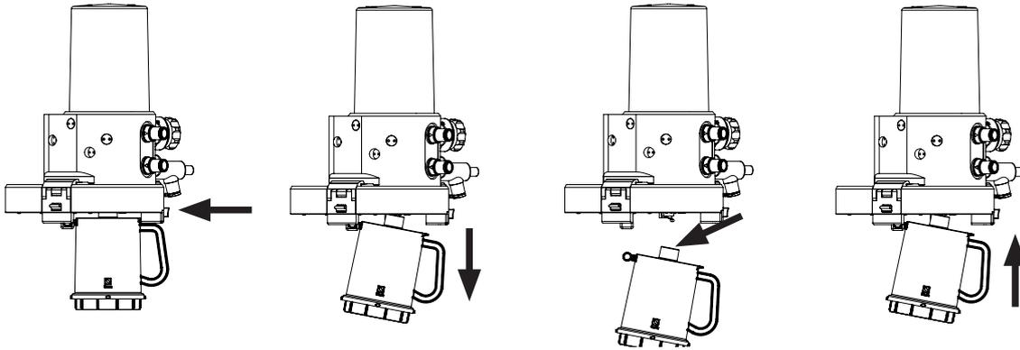
1. Press the button above the handle to release the absorber.
