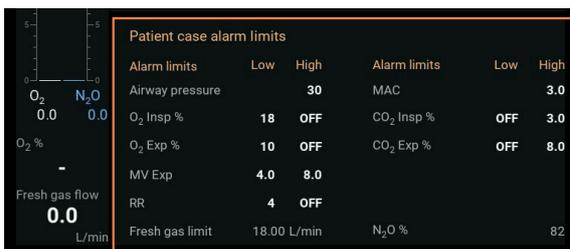
The values in this section relate to alarm limits for values measured by the machine during a procedure. The alarm limits are proposed settings based on the patient data entered (age and ideal weight). For details about setting alarm limits, see “Prepare a patient case” on page 42.
