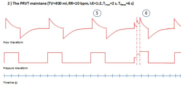
The pressure is applied as a constant pressure in the inspiratory phase of the breath. In the expiration phase, PEEP can be controlled to increase the handling of the lungs, by giving more optimal settings for the gas exchange.
