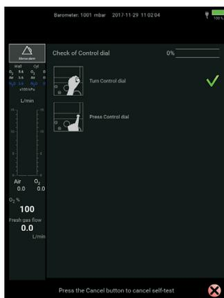
3. **Test of minoxygard.** During this test you will be asked to set and close the fresh gas flow accordingly. If the flow is not achieved a message will appear on the screen. Follow the instructions and repeat the test by pressing the Resume button.
