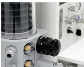
The APL valve is only active in MAN mode. Normally it is set between 5 and 20 hPa (cmH<sub>2</sub>O). Press the respiration bag to ventilate manually.
