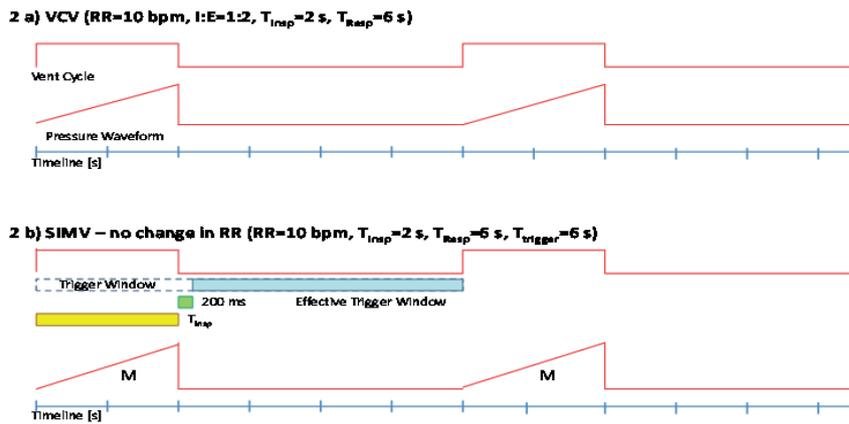
As long as the patient is triggering the ventilator in the trigger window, the patient is control. In case the patient is unable to trigger the ventilator, the mandatory breaths from the ventilator will secure that the patient gets sufficient ventilation due to the mandatory breath delivery. Should the patient again be able to trigger the ventilator, the patient can take control of the breathing.
