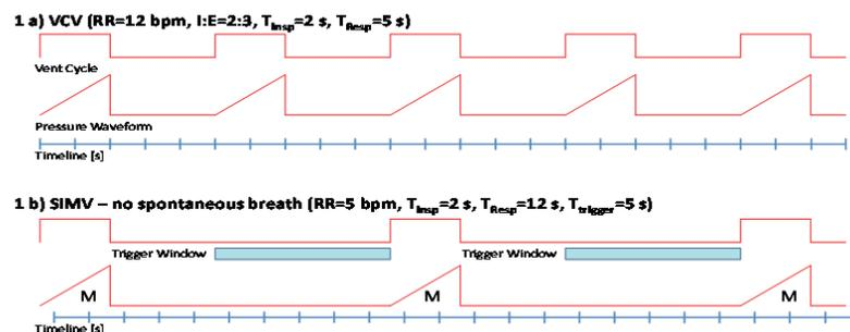
The trigger window is automatically calculated from the previous ventilation mode (one full breath = inspiration + expiration) using the available information:
