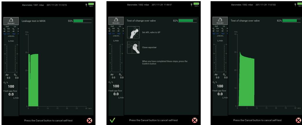
7. **Finalizing self-test.** The next sequences will show the result of the leakage test, prompt you to refresh gases in the breathing system and patient circuit, check the alarm sound, and prepare the machine for the first patient.
