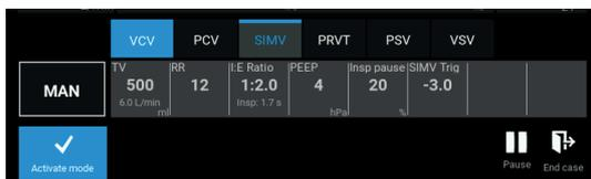
During a procedure you can select a different ventilation mode from the one currently used, and define settings for the new mode without affecting the current mode.
