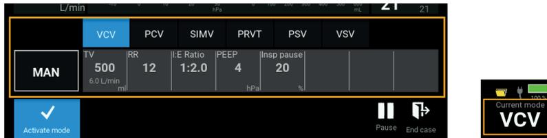
The currently active mode is highlighted in blue in the ventilation mode tab and shown in the *Current mode* field at the top right of the screen.
