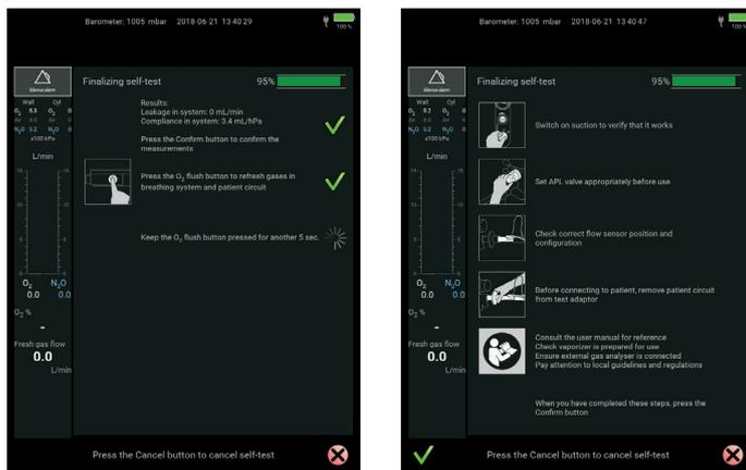
When the Full test has completed successfully, the machine returns to the Preparation screen.
