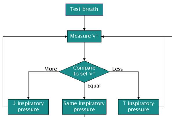
If there is a difference between the set tidal volume and measured tidal volume, the machine can calculate the needed inspiratory pressure to deliver the target tidal volume. This is possible as the system is calculating the Compliance.
