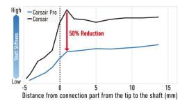
the tip to the joint of the shaft area enhances tracking ability.
