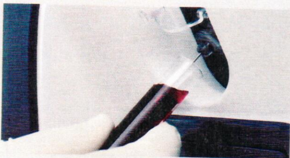
Samples can be aspirated directly from tubes. Sample transfer to a syringe or capillary is eliminated.
