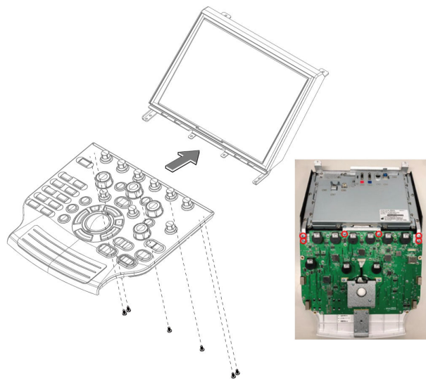
Figure 12-97 Disassembling OPIO Assy
