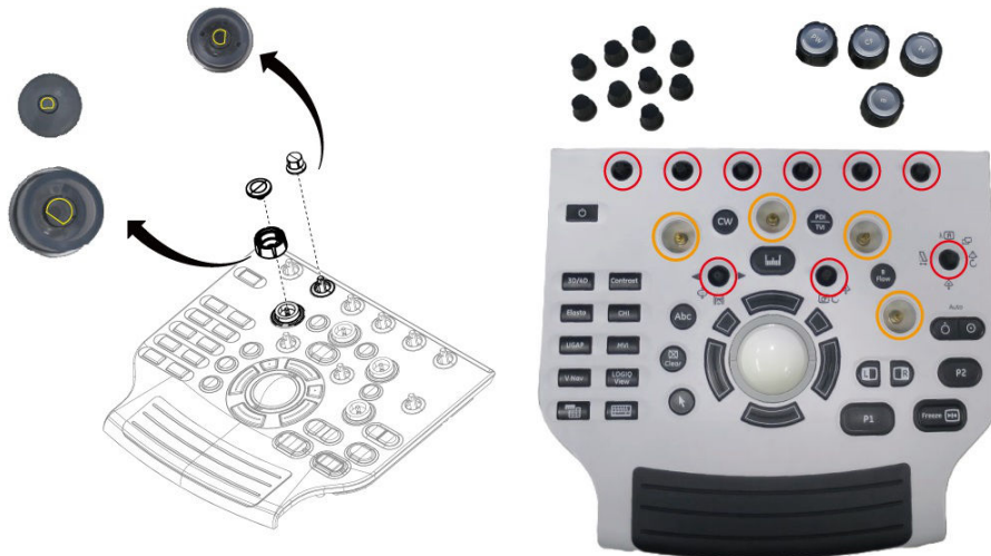
Figure 12-100 Removing OP knobs
