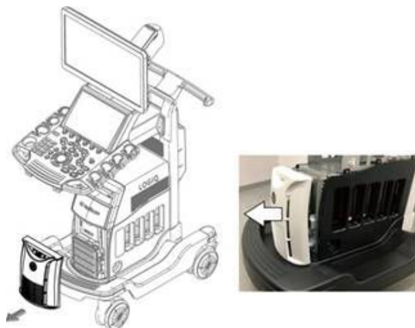
Figure 12-274 Removing front cover
