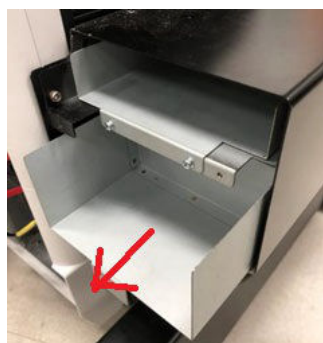
Figure 12-456 Removing LOWER BLIND TRAYS
