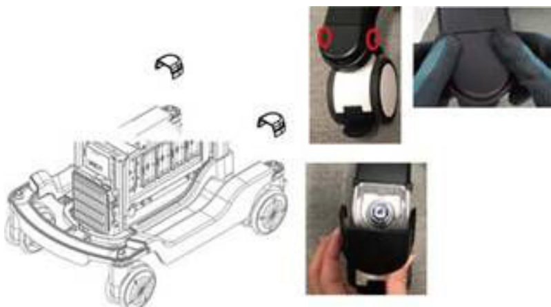
Figure 12-360 Removing base cover rear
