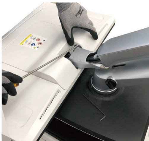
Figure 12-52 Removing the monitor cable cover
