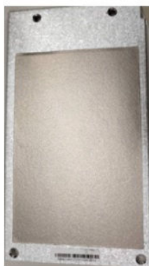
Power supply bracket cover with absorber sheet
