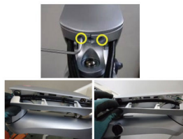
Figure 12-30 Removing 3rd Arm Cover
