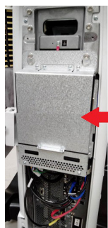
Figure 12-288 Removing Battery option
