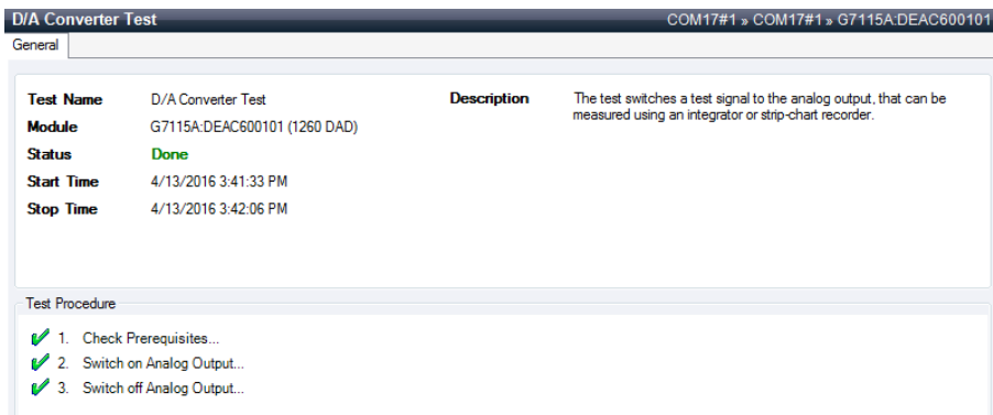
Figure 39: D/A Converter (DAC) Test – Results
