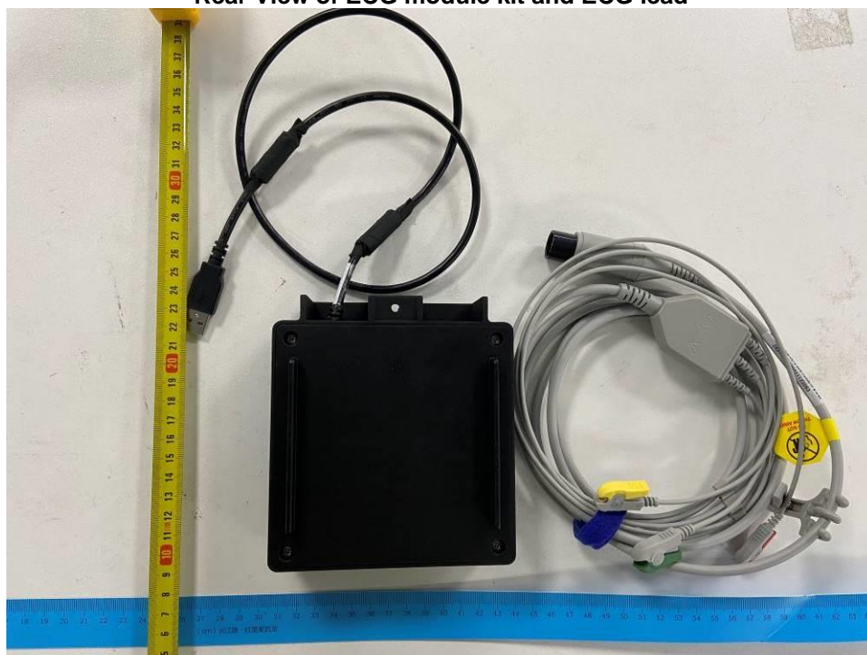
Rear View of ECG module kit and ECG lead
