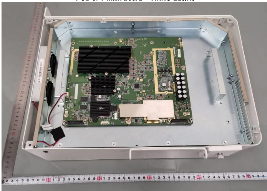
PCB of T-Main board – VINNO E20/X3
