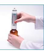
**Mounting:** Attach TLC sprayer to the bottle by turning anticlockwise. Never shake the sprayer during mounting.
