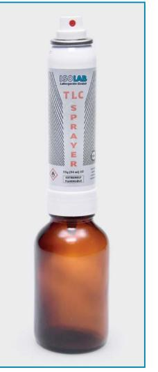
**Spraying:** Start spraying with the sprayer and release the button while the sprayer is still moving at the end of the TLC plate to avoid reagent loss. For best performance a spraying angle between 90° and 45° is required.
