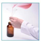
**Filling:** Pour the TLC reagent into the bottle. Never fill above the shoulder line.
