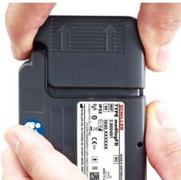
Remove/replace the external battery as follows:
