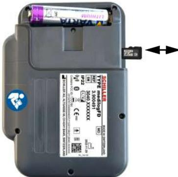
First, remove the recorder's battery cover to access the microSD card.
