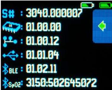
This menu displays specific recorder information, including the version and serial numbers of the recorder and other attached Bluetooth® devices/accessories. This information must be available when contacting Schiller service departments for help and troubleshooting.
