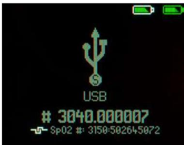
5. When the recorder is successfully connected to the PC, the following USB screen (left) is displayed on the recorder, including the recorder's serial number after the hash #. The recorder's serial number is also displayed on other medilogFD screens, including in the recorder's Info menu.
