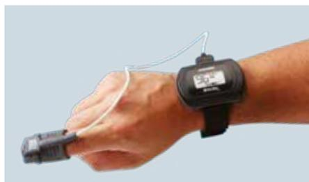
Wireless SpO<sub>2</sub> sensor, attached for the night
