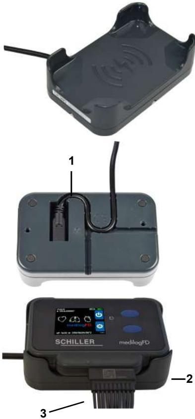
1. Connect the CS-3 to a suitable USB output of at least 10W **(1)**, e.g. using a power adaptor (optional accessory).
