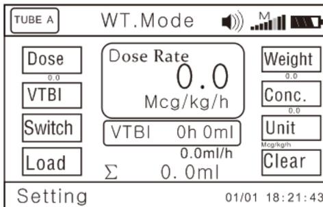
**Body Weight Mode (WT. Mode):** Press  for 'Dose' and input Dose Rate (0.1-2000).
