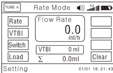
**Rate Mode:** Press  for 'Rate' and input rate value. Press ENTER key to save the value and exit to the previous menu.
