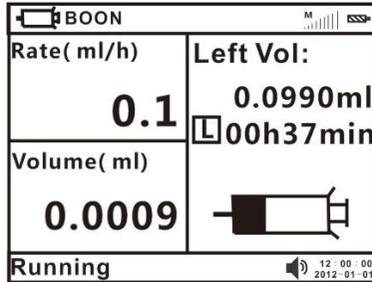
(Diagram17 Constant Flow Rate mode running interface)
