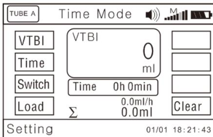
**Time Mode:** Press  for 'Time' and input time value. Press ENTER key to save the value and exit to the previous menu.
