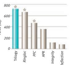
**Micromotion Test:** Micromotion testing demonstrated the importance of the Trilogy System's precise machining standards that result in a tight fit between the liner and shell. 16
