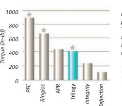
Lever-out testing proved the Trilogy System's resistance to high-torque exposure.
