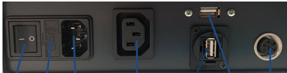
General ON / OFF switch Fuses box Cart power cord socket (not in use) Tri-polar jack for power cable supply USB connector, cart data connection (not in use) Connector for connecting the USB key Footswitch connector (not in use)
