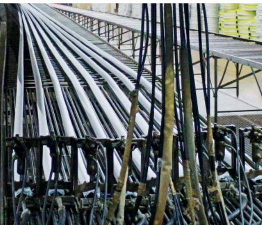
hoses during vulcanizing process
