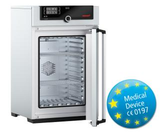
The indispensable safety feature for this hot air steriliser: Setpoint Wait. This means that the programme for sterilisation only starts when the set temperature has been reached. This feature can also be used with freely positionable Pt100 temperature sensors. Here the sterilisation time only begins when the set temperature has been reached at all measurement points, and reliable sterilisation is guaranteed at all times.
