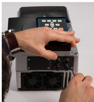
Fig. 36: Securing the M12 module
