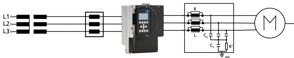
Fig. 31: Installing line choke and output filters
