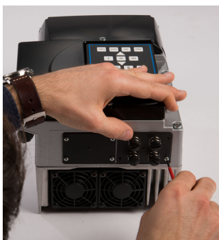
Fig. 43: Securing the M12 module
