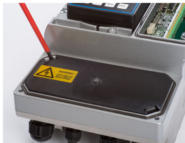
Fig. 13: Prying open the protective cover
