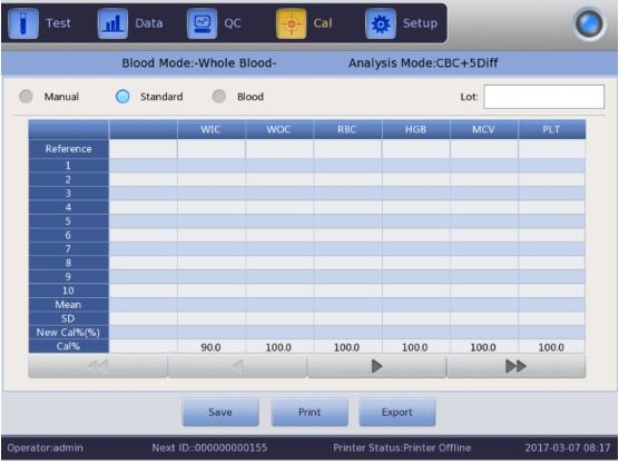
Figure 9-2 Standard Calibration
