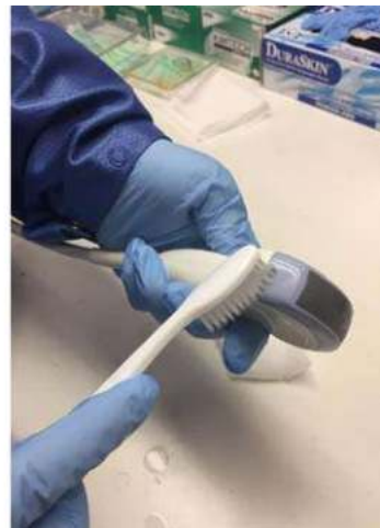
Figure 11-6. Cleaning the probe using a brush
