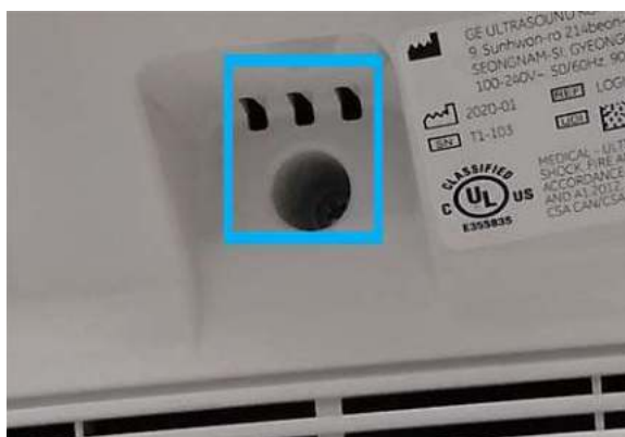
Figure 13-307. LED location of the battery
