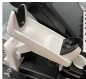
Figure 3-4. TVTR Probe Holder
