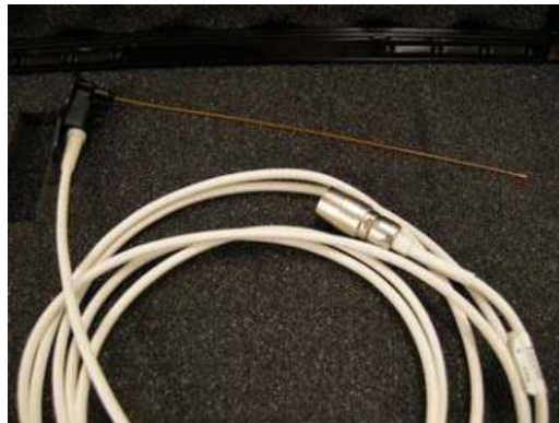
Figure 13-151. Needle Tip Sensor and Cable Close-up
