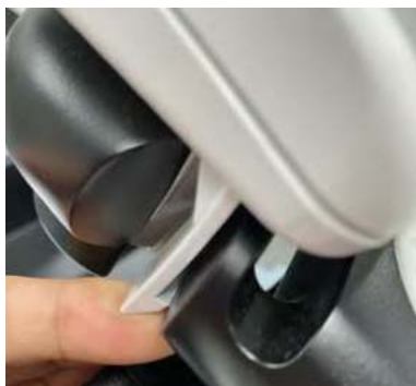
Figure 3-5. Pull the claw to remove
