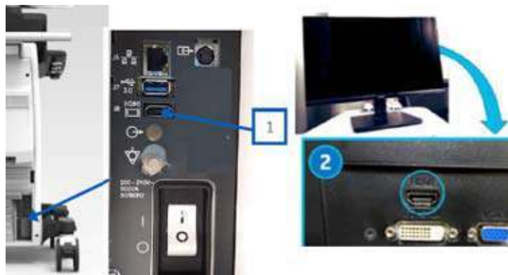
Figure 3-8. Connect HDMI Cable to back of LOGIQ Fortis and External Monitor
