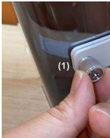
Figure 12-12. Screw of the storage tray
