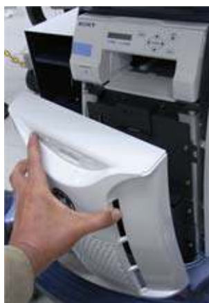
Figure 12-9. Remove the front cover
