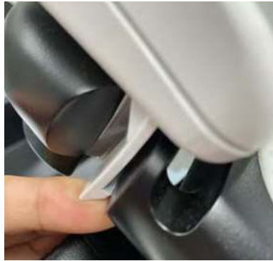
Figure 12-13. Pull the claw to remove
