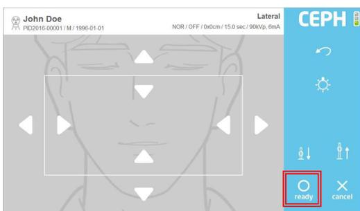
Press [ready] button after FOV adjustment on Console PC and/or the THU. The device moves to ready position for exposure.
