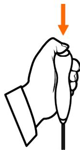
After the green light on the exposure switch has been illuminated, continue to press the switch until scanning has been completed.
