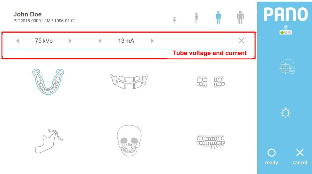
Fig 6 Exposure Condition Adjustment
