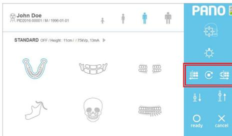
Adjust the position of Canine Beam by using touch screen or remote control.
