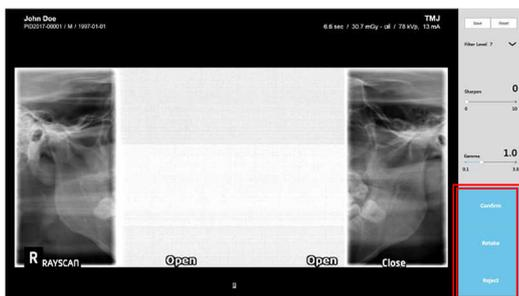
After scanning is completed, click [Confirm/ Retake/ Reject] buttons.
