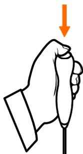
After green light on the exposure switch has been illuminated, continue to press the switch until scanning has been completed.
