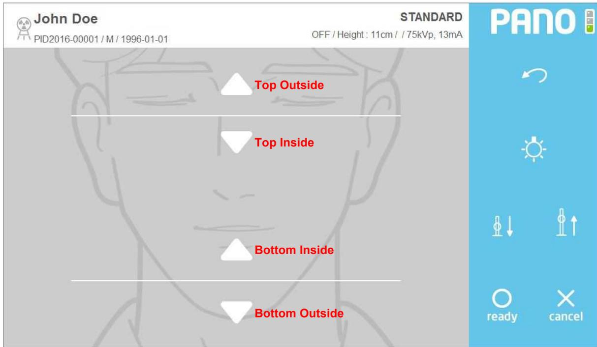
Fig 45 FOV Mode(Touch Monitor)
