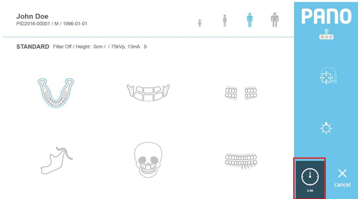
**Fig 8 Cooling Time Indicator**
