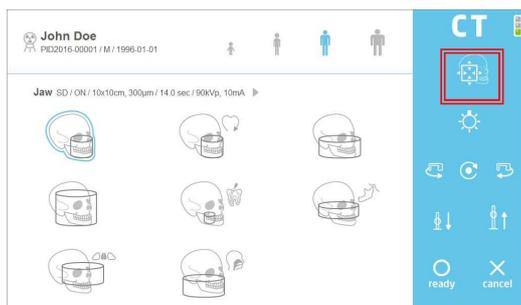
Use [FOV] button on the THU and/or remote controller to get into FOV Mode. Go to "8-2" if FOV adjustment not needed..
