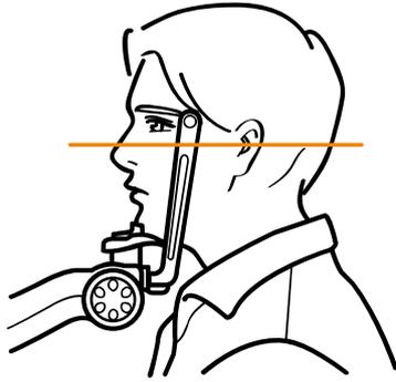
Use the horizontal alignment beam lever, mounted on the equipment Lift Column, to align the patient's Frankfort plane parallel to the laser.
