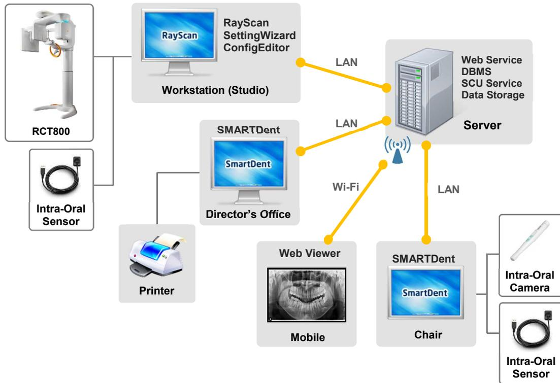
**Fig 55 System Configuration of RAYSCAN<sup>web</sup>**
