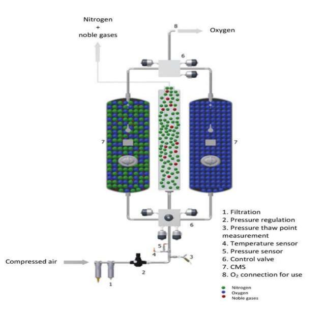
Through the Pressure Swing Adsorption (PSA) technology and adsorption media developed in-house, the atmospheric air is separated in its components nitrogen and oxygen. Subsequently, oxygen is available for further use in quantities of 0.5 - 2.000,00 Nm<sup>3</sup>/h and purities of 90.0 - 95%.
