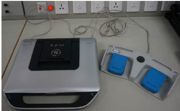
Figure 3-5. Connect Footswitch to the system
