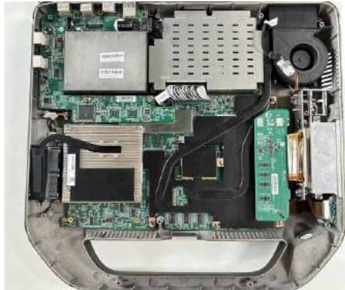
Figure 8-8. MST board installed
