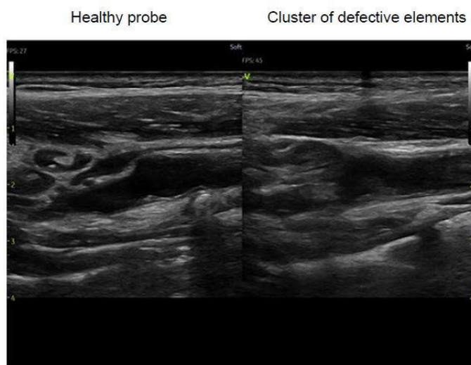
Figure 7-63. Example of image degradation for a linear probe
