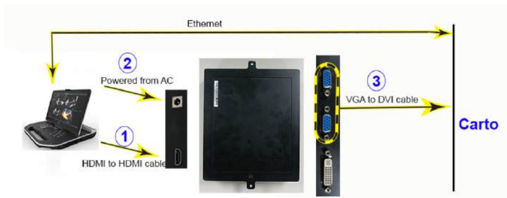
Figure 3-153. Vivid iq interfacing with the CARTO® 3 - Protocol 1.0
