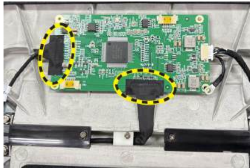
Figure 8-6. Stick the acetic acid tape
