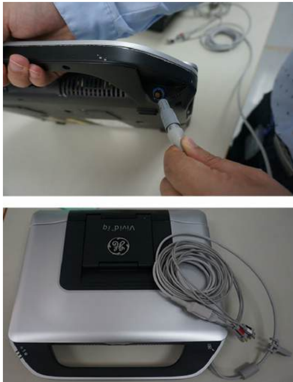
Figure 3-6. Connect ECG to the system
