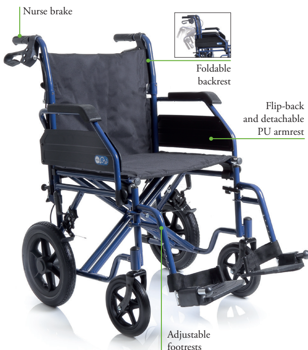
CP520 series Double cross, rear solid tires, folding backrest
