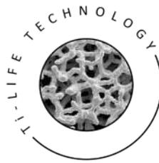
The structure mimics the bone trabecular geometry and is designed to allow bone in-growth. This technology is based on a propriety algorithm associated with a unique additive manufacturing process, commonly referred to as 3D printing.
