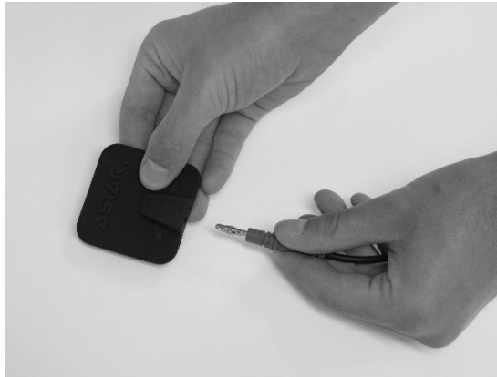
Figure 3.2. Connection of electrodes
