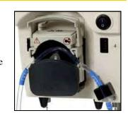
Assure that the clips on ends of the raceway are lined up with the tube segment.
