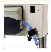
Plug the transducer connector marked 4 on the Infusion Set into the pressure transducer receptacle (labeled 4) on the front of the Console. Ensure that the connector is fully seated.
