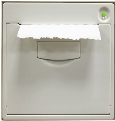
Figure 2-10 Installing Thermal Paper (3)
