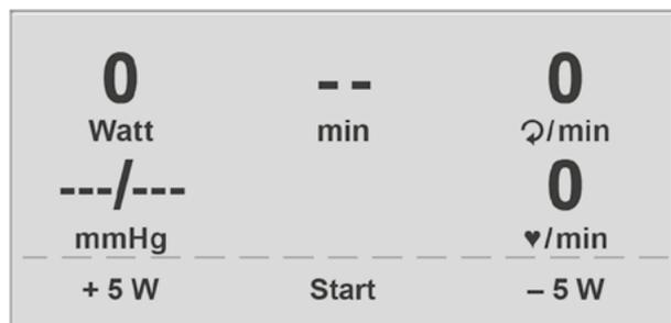
Figure 8-14: Initial screen of a manual exercise test
