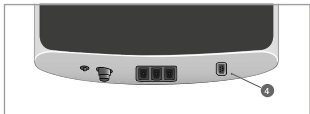
Figure 4-13: SpO2 sensor connection
